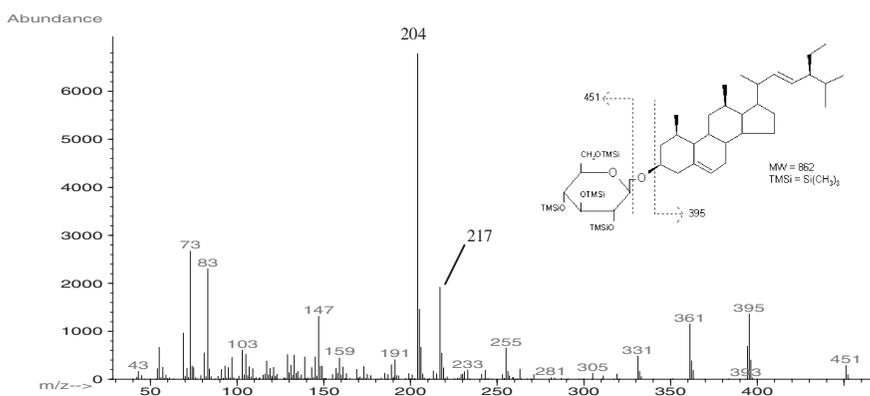
FIG. 3. MASS SPECTRUM FOR TRIMETHYLSIYL ETHER DERIVATIVE OF STIGMASTERYL GLUCOSIDE IN SOYBEANS (2, FIG. 1B)
