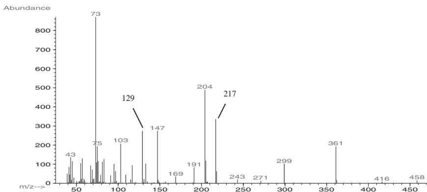
FIG. 6. MASS SPECTRUM FOR LATE ELUTING PEAK IN WHOLE WHEAT FLOUR DISPLAYING TRIMETHYLSILYL GLUCOSE DERIVATIVE (5, FIG. 1D)
