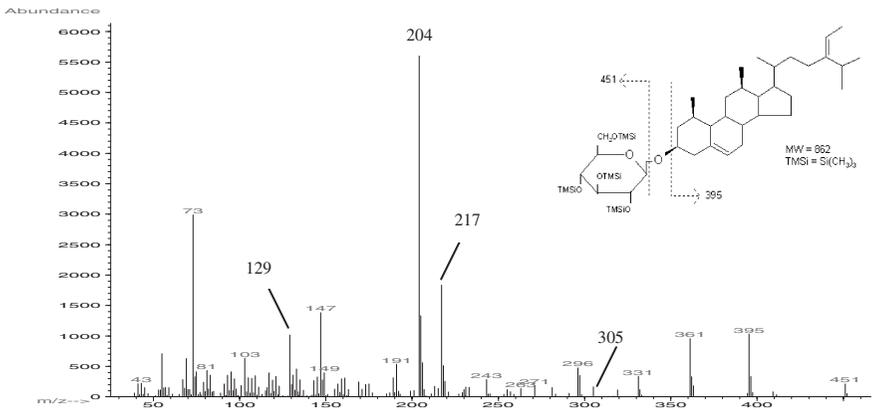
FIG. 5. MASS SPECTRUM FOR TRIMETHYLSILYL ETHER DERIVATIVE WITH PRESUMPTIVE IDENTIFICATION OF  $\Delta^5$ -AVENASTERYL GLUCOSIDE IN GRANOLA BAR (4, FIG. 1C)
