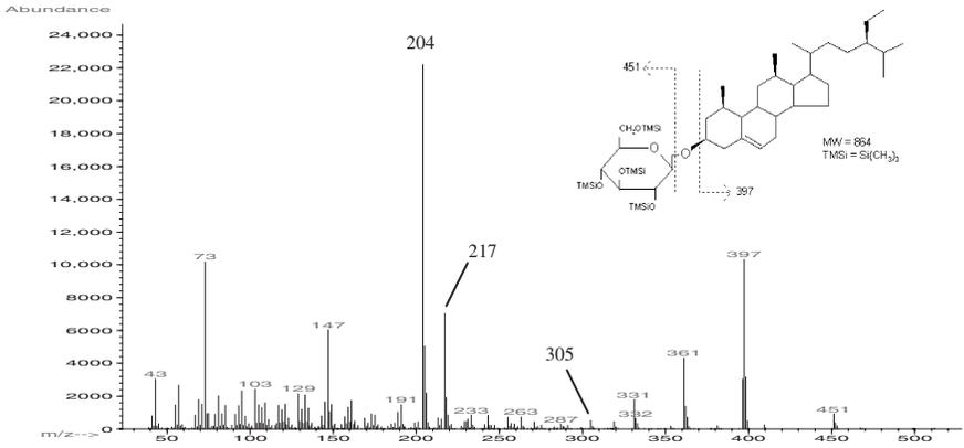
FIG. 4. MASS SPECTRUM FOR TRIMETHYLSILYL ETHER DERIVATIVE OF SITOSTERYL GLUCOSIDE IN SOYBEANS (3, FIG. 1B)
