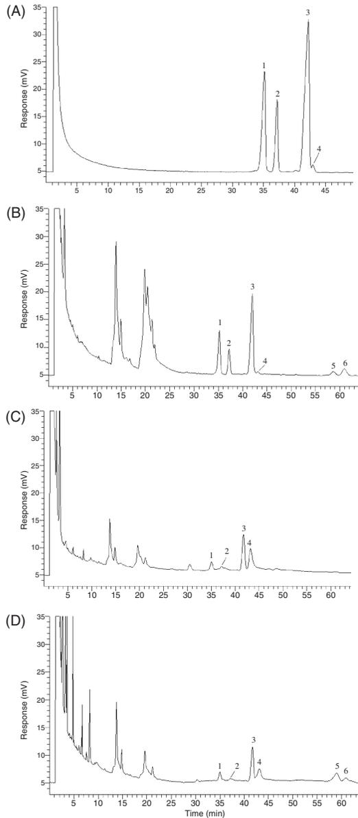
FIG. 1. REPRESENTATIVE GC-FID CHROMATOGRAMS FOR STERYL GLUCOSIDES IN (A) STANDARD MIXTURE, (B) SOYBEANS, (C) GRANOLA BAR AND (D) WHOLE WHEAT FLOUR
